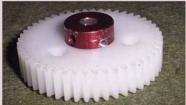
This shot shows the original mounting hole (on the left) next to the newly drilled hole. The new hole is partially hidden by the white gear wheel
