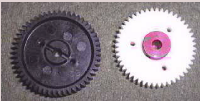
Here's the original idler gear next to the Vario replacement. The red part on the Vario gear is the separate hub
