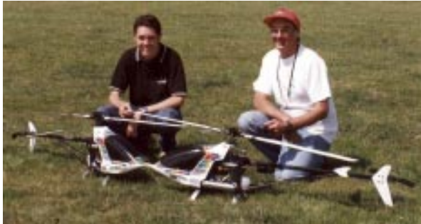
Just one of these will set you back about £3000! Peter and Mark Christy with their two Hirobo Eagle II EX competition machines, both use JR radio and the OS61SX-H WC engine running on 20% Formula Irvine fuel. JR 3000 piezo gyro, 2700 tail rotor servo, and a 4000 on the collective. Below: Peter calling for Mark during one of the hovering manoeuvres
