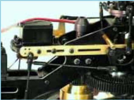
Above, Left side collective arm Swashplate and mixing levers shown below
