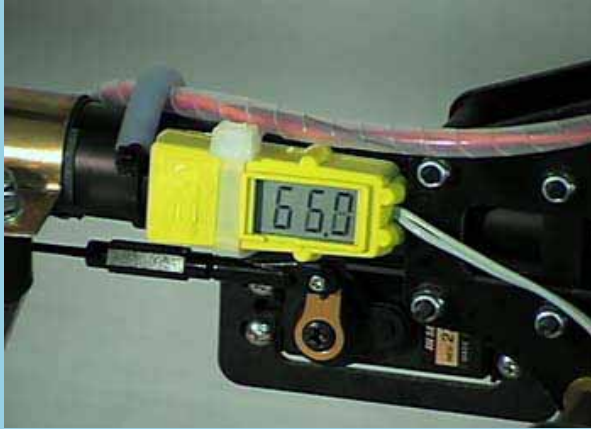
MIP temperature gauge to track engine temperature
