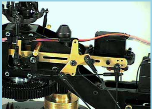
Rotor head with adjustable Bell-Hiller mixing
