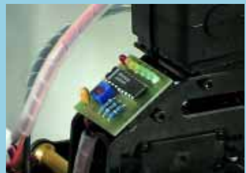
On board battery monitor
