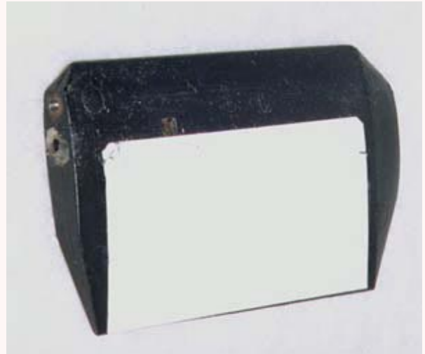
The standard Hirobo Shuttle ZX paddle. Note the weight in front of the mounting hole. This thick, 25 gram paddle works well for most type of flight.
