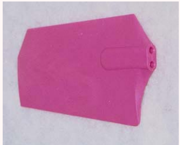
K&S of Japan 30 size dual rate flybar paddle #328. Note the two mounting holes. The forward hole is for less cyclic speed relative to the rear mounting. This thin, light (16 gram) paddle can radically change the cyclic rate of your heli. Taming it with adjustable flybar weights may be desirable on some head designs (Ed: Desirable! I'd say vital... :-)
