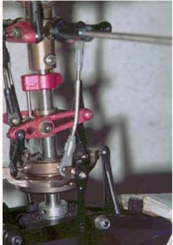
The ARK floating swashplate system on an upgraded Shuttle ZX. Note the swashplate is designed to move up and down the mainmast and the washout only has one mixing arm on each side.
