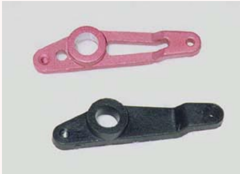
The stock Shuttle ZX plastic seesaw arms and the ARK metal units with machined bearing seats. The plastic unit accepts a flanged bearing on each side of it therefore it will take a long time before the bearing seats show any compression wear.
