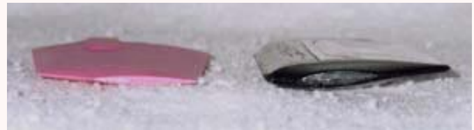
An end view of the ZXX and K&S paddles. Note the differences in airfoil and thickness.
