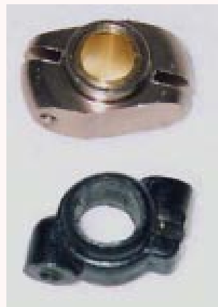
The stock plastic washout hub from Shuttle and the ARK 5203-042 Machined Metal Washout Hub - note the bronze bush in the center to ride up and down on the mainmast and to take the mixing loads.
