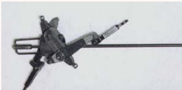
The collective mechanism only from Photo #6. Note the long Center Control Rod and the two outer rods that come back and attach to the washout, and the complexity of the four mixing arms used.
