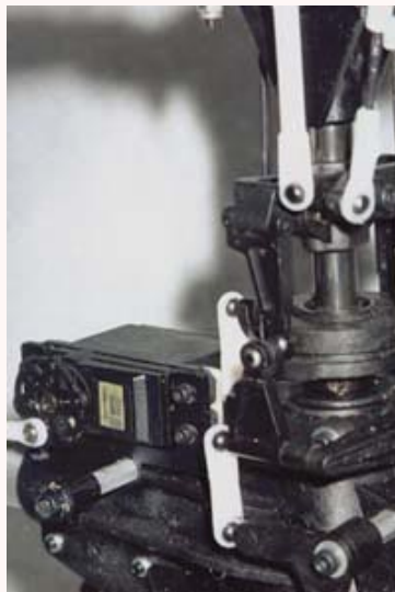
The fixed swashplate system of the Kalt Enforcer / Space Baron.
