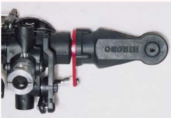
The underside of the stock Shuttle ZX seesaw unit. Note the thickness of the bearing seat area of the control arms allowing for a bearing on each side with spacers between them. A well designed plastic arm.
