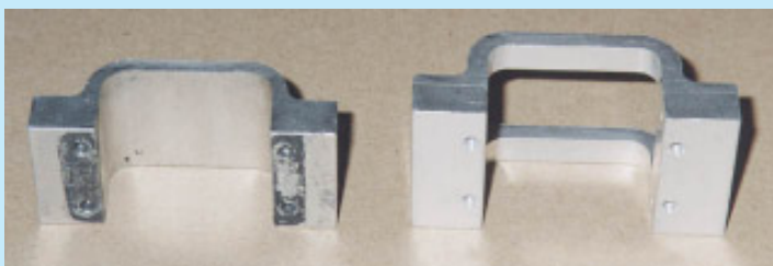
Photo #7 - The Shuttle one-piece motor mount (left) and the Hawk one-piece unit (right) with the back machined out to save weight.
