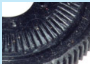
Photo #12B - An X-Cell 60 stock molded plastic main gear with the stripped T/R drive teeth molded on the top. They also come with a set of T/R drive teeth on the bottom.
