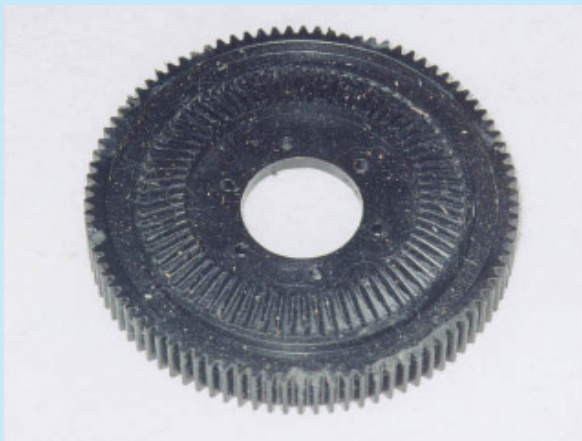
Photo #12B - An X-Cell 60 stock molded plastic main gear with the stripped T/R drive teeth molded on the top. They also come with a set of T/R drive teeth on the bottom.
