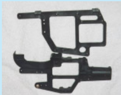
Left, photo #4 - View of the plastic molded bearing seats of the Shuttle sideframe and right, photo #5 - The two piece molded plastic "stacked" frame design of the Century Hawk
