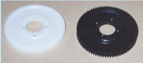
Photo #12 - Two main gears for the TSK Mystar 30. On the left is the unnecessary upgrade CNC machined nylon unit and on the right is the stock molded reinforced plastic unit.
