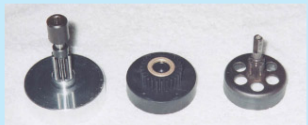
Photo #11 - Various Clutch bells - (from left) Machined Aluminum TSK Mystar 60 unit with built in one-way bearing hex start system, the plastic Century Hawk unit molded onto the steel pinion gear and the stamped aluminum Hirobo Shuttle Z unit that is pinned/welded to the pinion.
