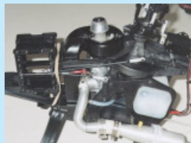
Photo #3 - Molded plastic modular sideframes of Kalt Enforcer/Space Baron
