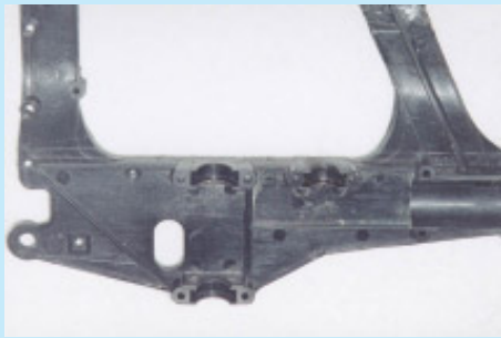
Left, photo #4 - View of the plastic molded bearing seats of the Shuttle sideframe and right, photo #5 - The two piece molded plastic "stacked" frame design of the Century Hawk
