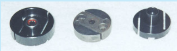
Photo #10 - Machined one piece metal clutches - (from left) TSK Mystar 60, X-Cell 60, Century Hawk
