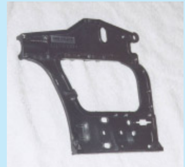
Photo #2 - Molded plastic one piece Hirobo Shuttle side frame
