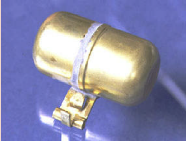
A float from an old Ford carburettor, above in its original form and below, with the air vent pipe attached. So far it's worked well in use
